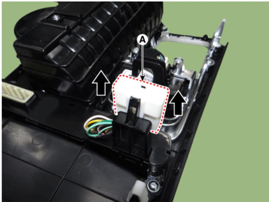
5. Loosen the screw and then remove the console floor switch complete (A).
