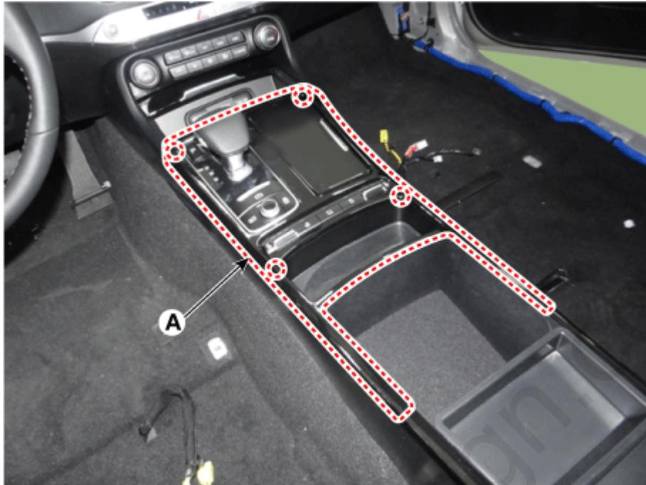
3. Disconnect the connector (A) from the console upper complete.
