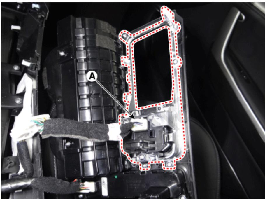
8. Disconnect the ESP connector (A) from the upper console.
