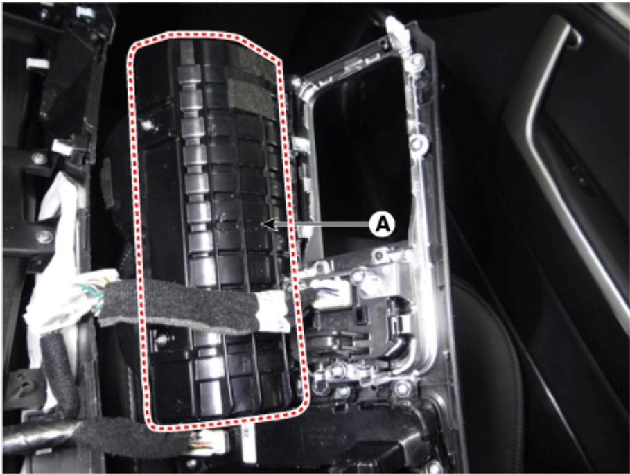
7. Loosen the screw and then remove the ESP switch (A).
